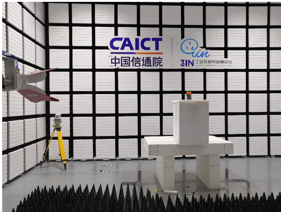
Description: Radiated Emission Test Setup (1GHz -18GHz)
