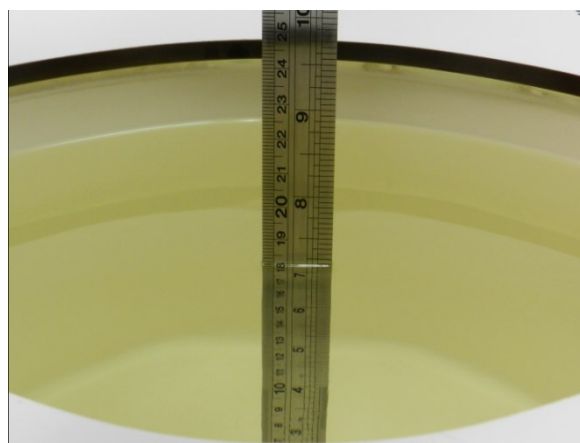
Fig 11.1.2 Photo of Liquid Height for Body SAR
