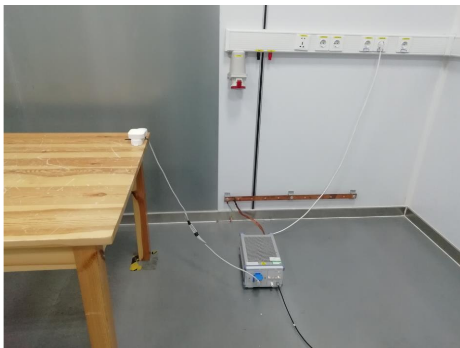
Fig. 4 Power line conducted emission setup photo
