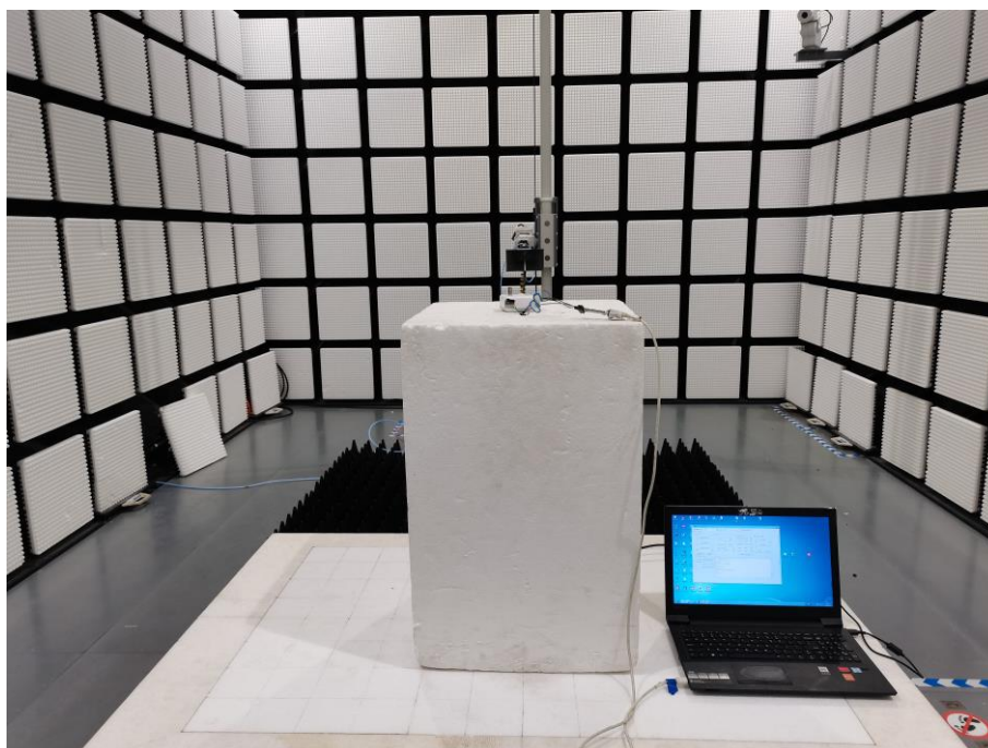
Fig. 3 Radiated emission setup photo(Above 1GHz)
