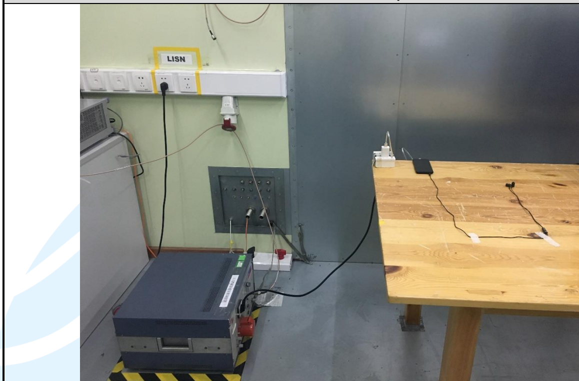
Conducted Emission Test Setup - Mode 2
