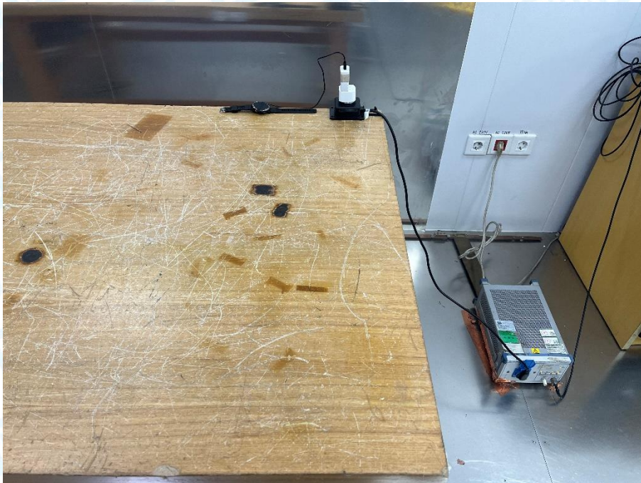
Photo of Setup for Radiated Emission (30MHz~1GHz)
