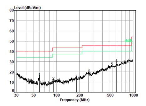
Site : chamber Condition: 3m VERTICAL Job No. : 00927ET Test Mode: 00
