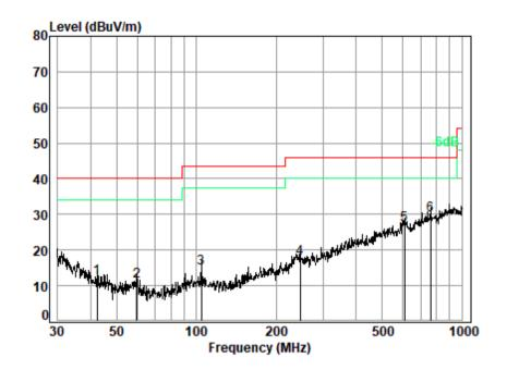
Site : chamber Condition: 3m HORIZONTAL Job No. : 00927ET Test Mode: 00
