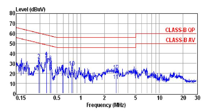
Site : conducted #1 Date : 02-24-2017 Condition : CLASS-B QP LISN : NEUTRAL Tem / Hum :  $18 \, ^{\circ}\text{C} \, / \, 60\%$  Test Mode : CH+OP Mode
