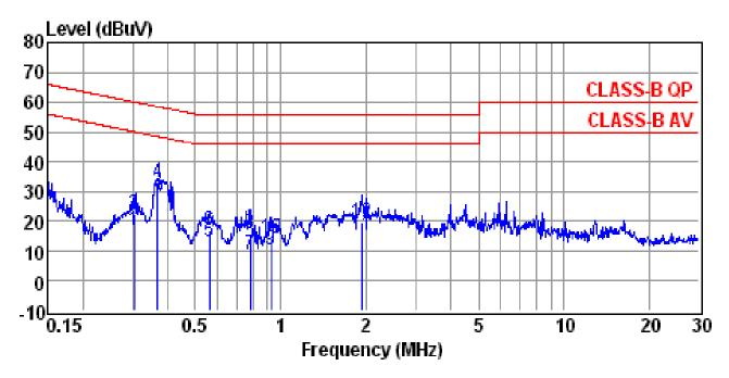
Site : conducted #1 Date : 12-08-2016 Condition : CLASS-B QP LISN : NEUTRAL Tem / Hum :  $22 \,^{\circ}\text{C} \, / \, 61\%$  Test Mode : BT Mode
