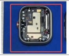
The antenna is Metal mid-frame antenna.
