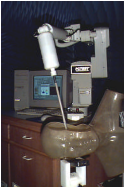
Figure 5. Photograph of the Probe and the Phantom
