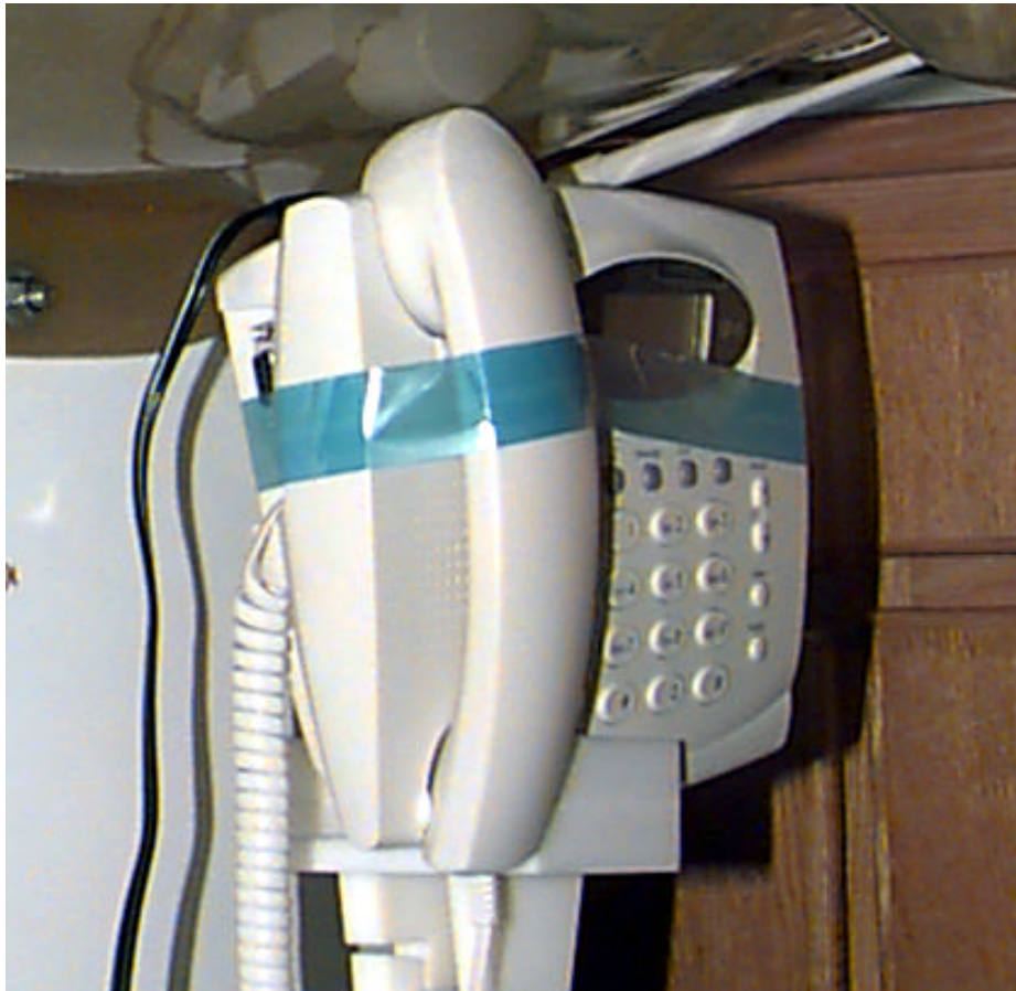
Figure 8. Test setup of EUT in normal operating position with the source of significant emissions (antenna) 2.0 cm below the phantom.
