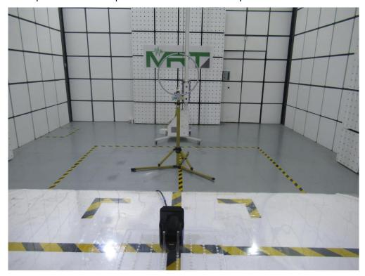
Mode 2  $\label{eq:Description:Radiated Spurious Emission Test Setup for 30MHz $\sim 1$GHz }$
