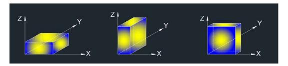
Note 1: For radiated test, EUT in each of three orthogonal axis emissions had been tested, but only the worst case (X axis) data recorded in the report.
