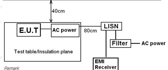
EUT: Equipment Under Test LISN: Line Impedence Stabilization Network Test table height=0.8m
