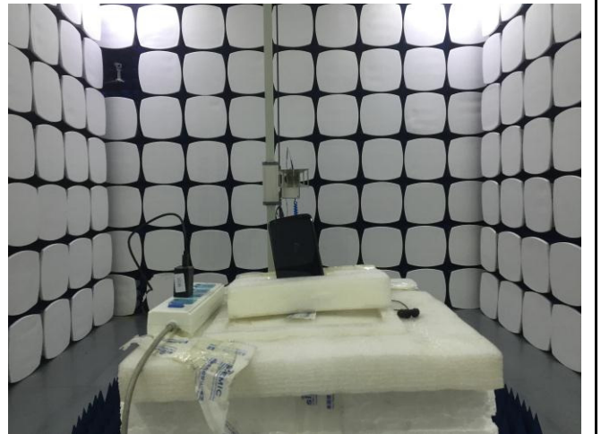
Radiated Spurious Emissions Test Setup Above 1GHz
