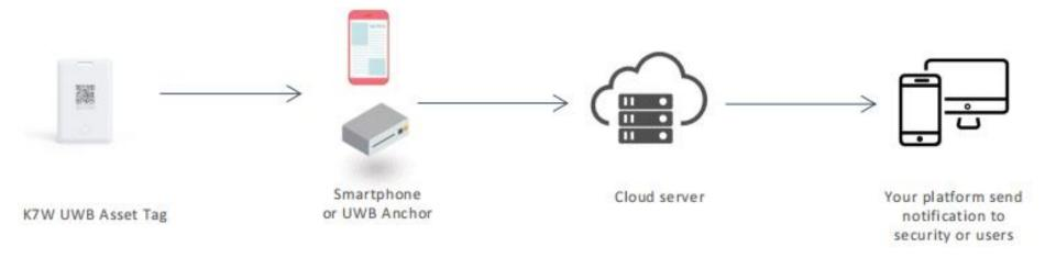
Using the app/UWB Anchor to scan/connect the K7W' signal, then the APP/Anchor receivd its data and handle the data to reach the location usage.
