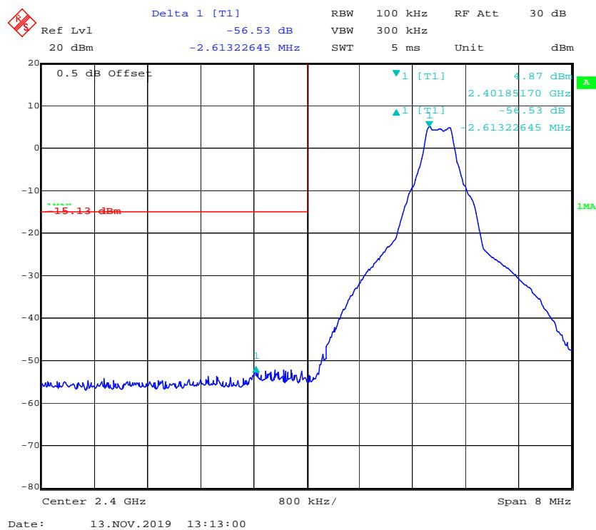
**Band Edge, Right Side**
