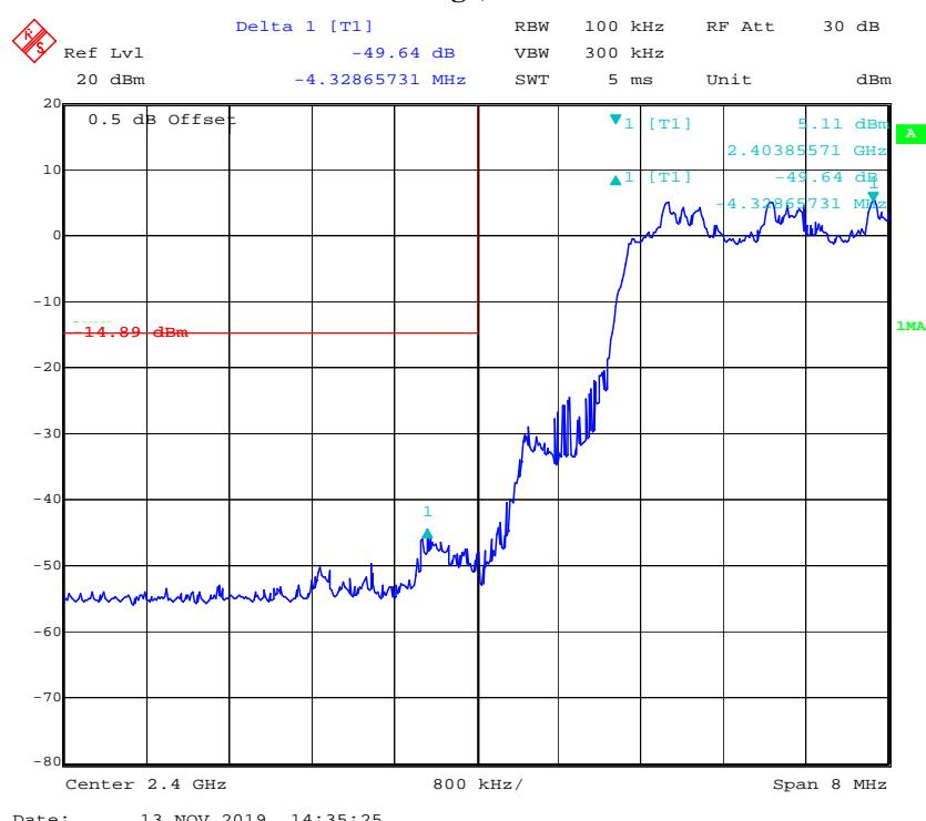
**Band Edge, Right Side**
