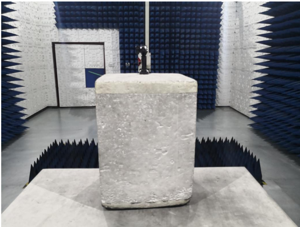
FCC RADIATED EMISSION TEST SETUP ABOVE 1GHZ
