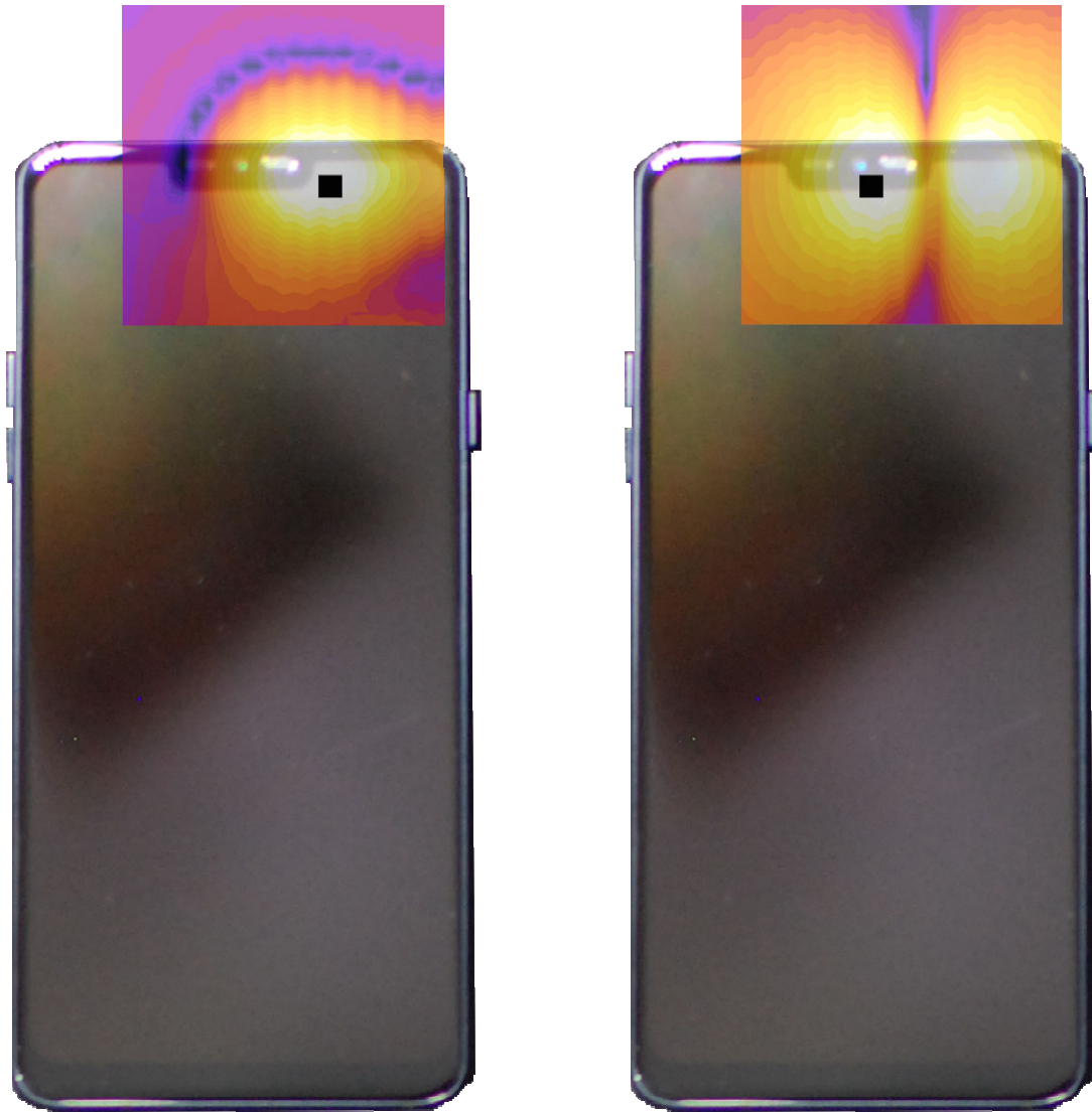
Figure 16-3 T-Coil Scan Overlay Magnetic Field Distributions
