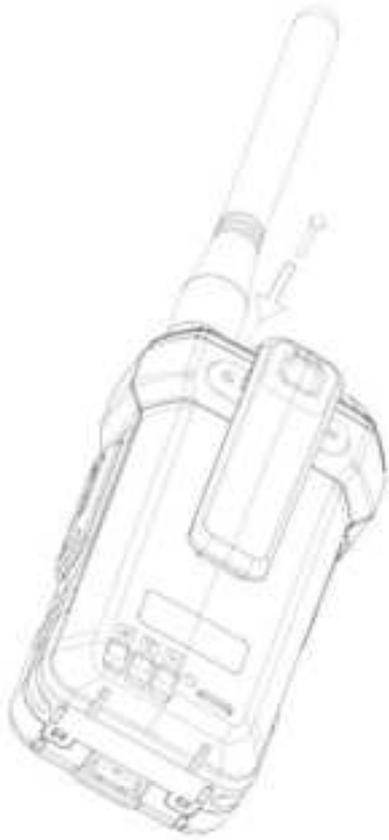
Place the belt clip to the corresponding grooves on the back of the radio, and then screw it if need. Anticlockwise turn screws to remove the belt clip.
