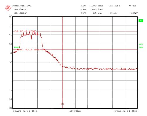
According to document [3] part G2d the measured field strength was converted to EIRP and compared to the limit of -17 dBm/MHz (within the frequency range from the band edge to 10 MHz above or below the band edge):
