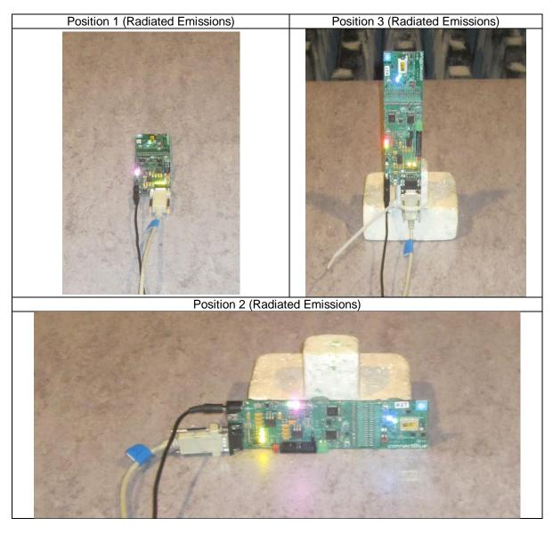
Preliminary tests were performed to find worst-case configuration and position. The radiated emission measurements were carried out in the orthogonal direction that emits the highest spurious emission levels.
