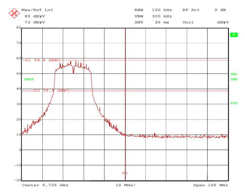
According to document [3] part G2d the measured field strength was converted to EIRP and compared to the limit of -27 dBm/MHz:
