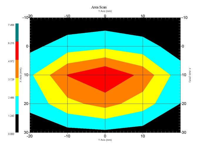
1 gram SAR value : 5.292 W/kg 10 gram SAR value : 2.637 W/kg Area Scan Peak SAR : 6.215 W/kg Zoom Scan Peak SAR : 10.080 W/kg
