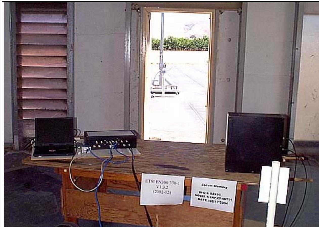
Radiated Emissions - Back View with Mag Loop Antenna
