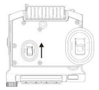
4 Align the concave side of the plastic upper cover with the aluminum chassis, and then press the cover until the latches are properly locked.
