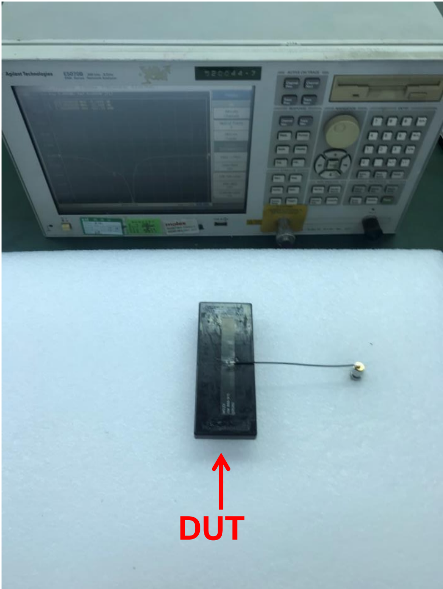
FIGURE4.1.2 ANTENNA LOADED WITH PC/ABS BLOCK OF 2MM THICKNESS TESTED WITH VNA E5071C
