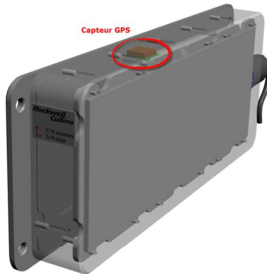
Figure 109: GPS antenna position on the PSR-500 radar
