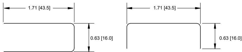
Mounting in cut-out in sheet metal (thickness 0.7 mm to 1.0 mm)
