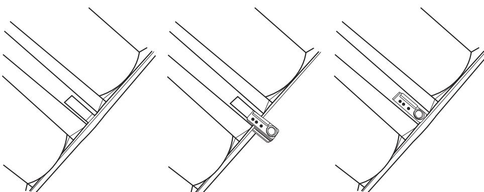
Mounting in a cut-out with mounting bracket
