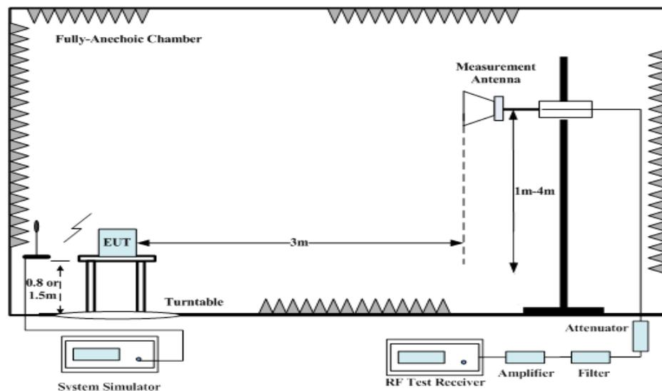
2. The EUT is then put into continuously transmitting mode at its maximum power level during the test and the maximum value of the receiver should be recorded as (Pr).
