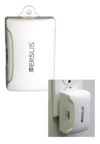
The Link combines both sets of information into a data packet that it transmits via the 2.4 GHz RF signal to the V-Link Gateway. The Links communicate over a two-way wireless RF channel in the 2.4GHz spectrum, secured by an encryption algorithm. The proprietary, patented V-Link communication protocol is designed to co-exist with other networks and will not interfere with existing IEEE 802.1x signals (i.e. Wi- Fi, ZigBee).
