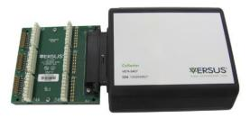
A punch-down connector block is included with each Collector. The connector block plugs directly into the 50-pin Amphenol connector on the side of the Collector. Up to 4 Collectors, including the internal Collector within the VER-2037 Concentrator, can be connected from one to another in a daisy-chain configuration.
