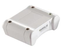
The Gateway communicates over a two-way wireless RF channel in the 2.4GHz spectrum, secured by an encryption algorithm. The proprietary, patented V-Link communication protocol is designed to co-exist with other networks and will not interfere with existing IEEE 802.1x signals (i.e. Wi-Fi, ZigBee).
