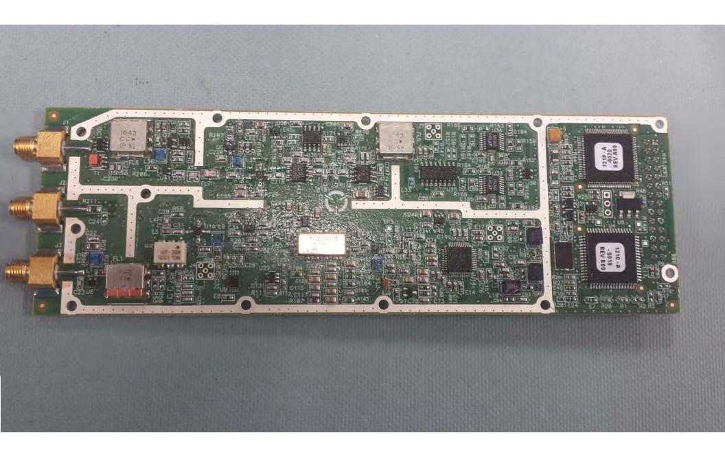
BGAN RF Card - Top (removed from piggyback, cover off)
