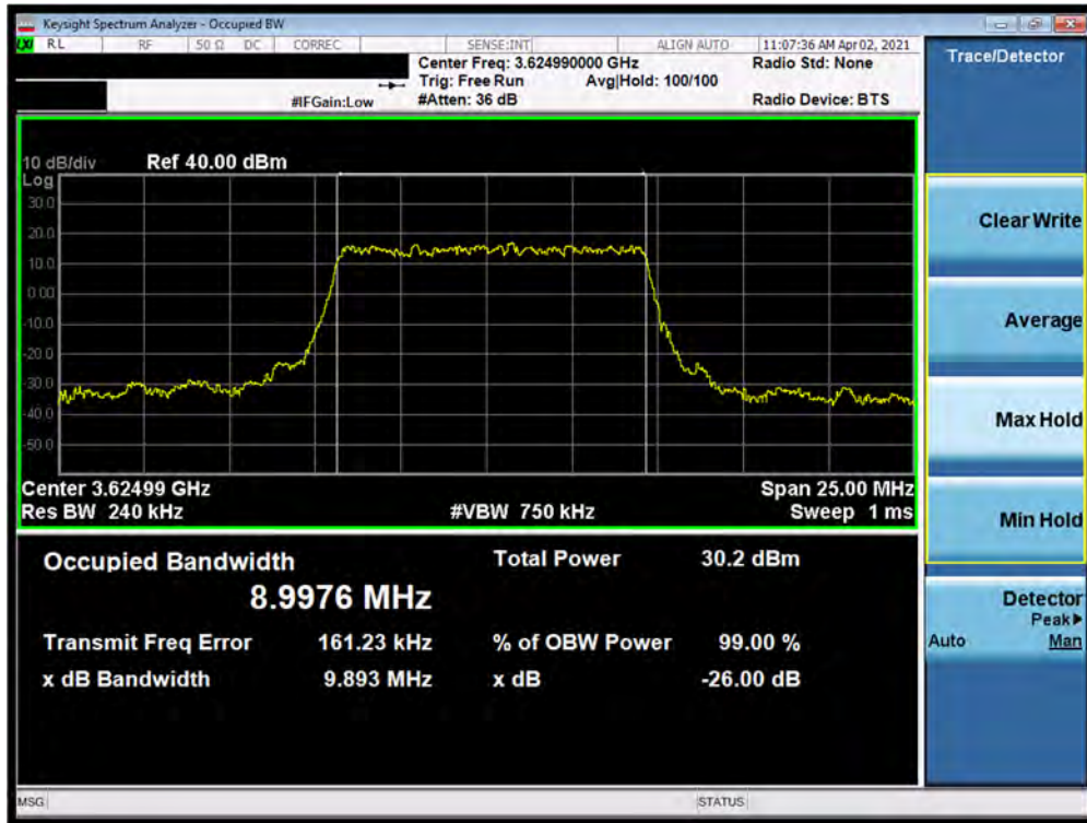
Plot 7-7. Occupied Bandwidth Plot (NR Band n48 - 10MHz \pi/2 BPSK - Full RB Configuration)
