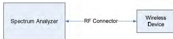
Figure 7-1. Test Instrument & Measurement Setup
