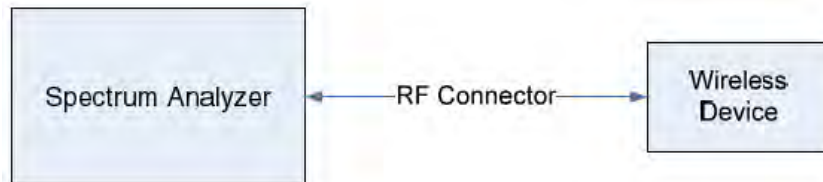
Figure 7-4. Test Instrument & Measurement Setup
