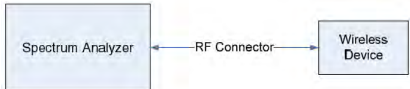
Figure 7-3. Test Instrument & Measurement Setup
