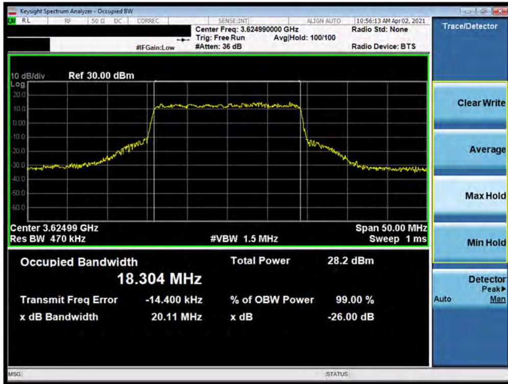
Plot 7-5. Occupied Bandwidth Plot (NR Band n48 - 20MHz QPSK - Full RB Configuration)
