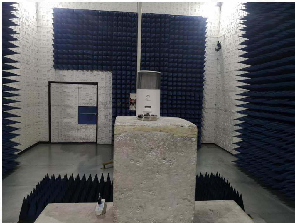
FCC RADIATED EMISSION TEST SETUP ABOVE 1GHZ
