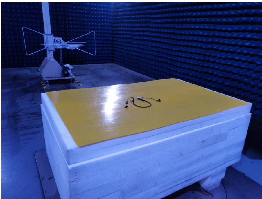
Photo of Radiated Emission Measurement (Above 1G)
