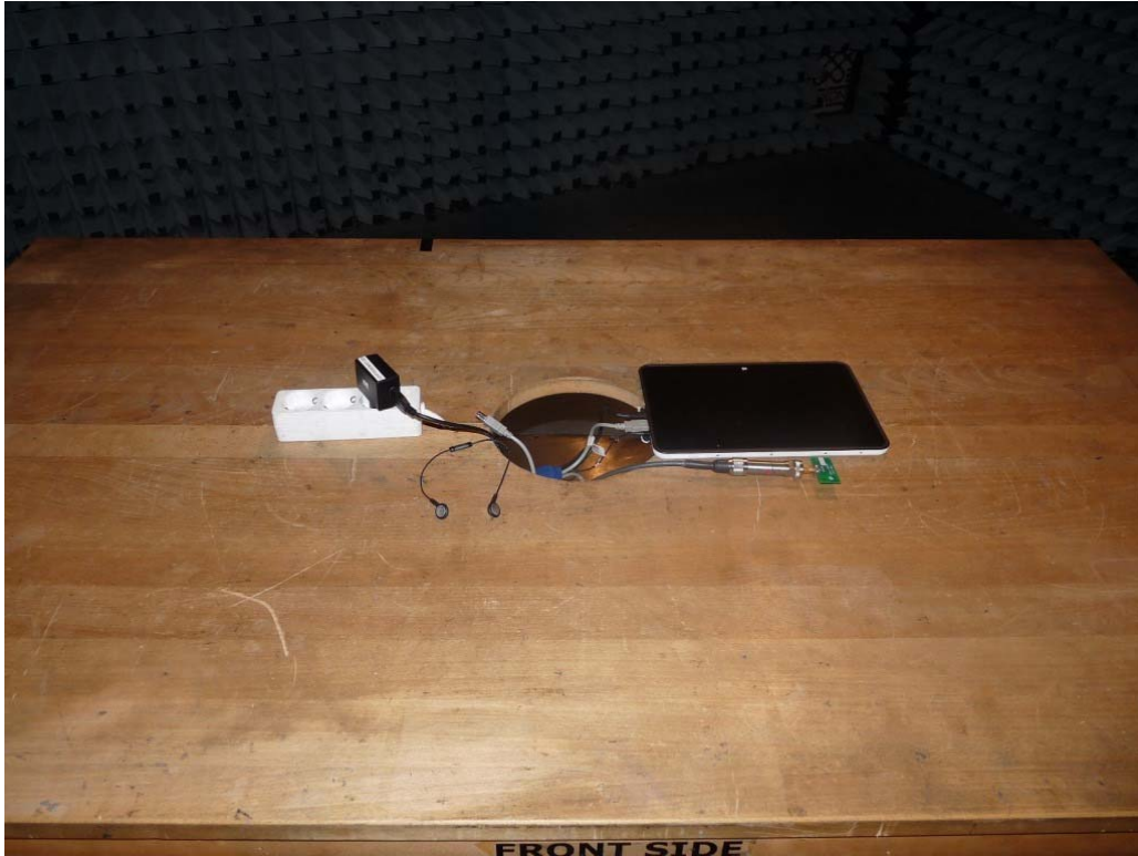
Photo 3: Test setup for radiated measurements (AC Port (power line), EUT supplied by battery, unintentional radiator §15)
