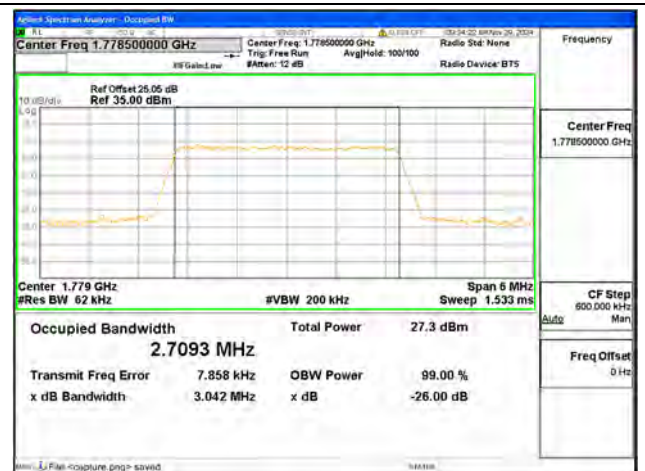
B66 / 3MHz / 64QAM/ High CH
