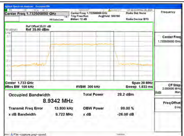
B4 / 10MHz / 16QAM/ Mid CH
