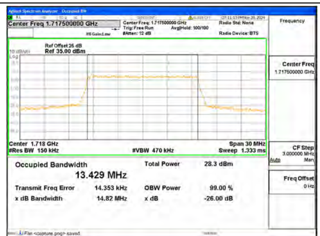
B4 / 15MHz / 16QAM/ Low CH
