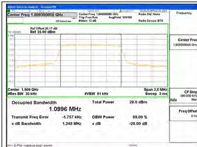
B2 / 1.4MHz / QPSK/ High CH
