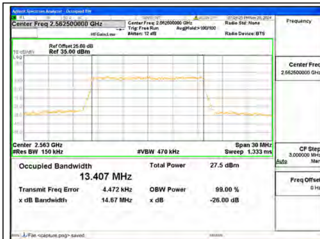
B7 / 15MHz / QPSK/ High CH
