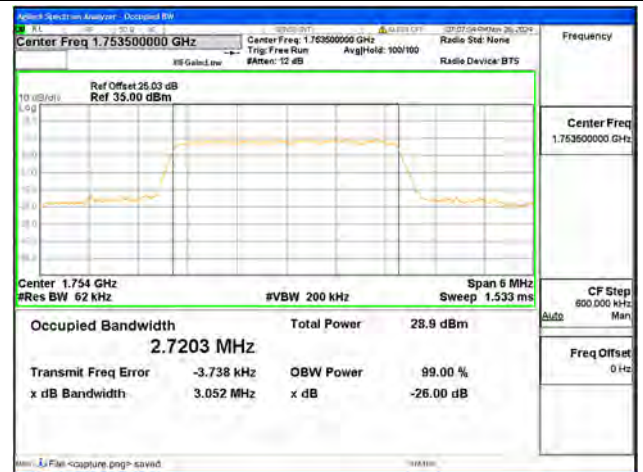
B4 / 3MHz / QPSK/ High CH
