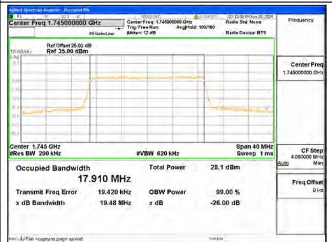
B4 / 20MHz / 64QAM/ High CH
