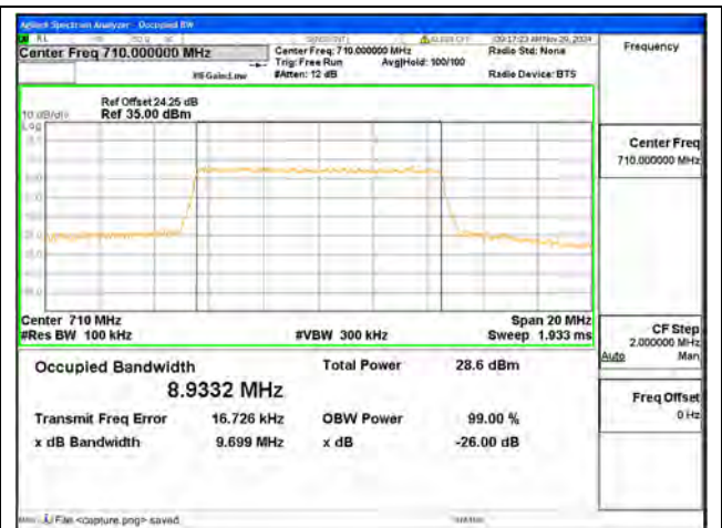
B17 / 10MHz / 16QAM/ Mid CH
