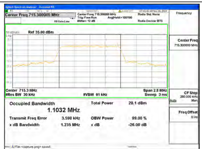
B12 / 1.4MHz / 16QAM/ High CH
