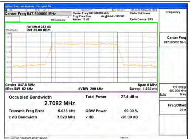
B5 / 3MHz / 16QAM/ High CH
