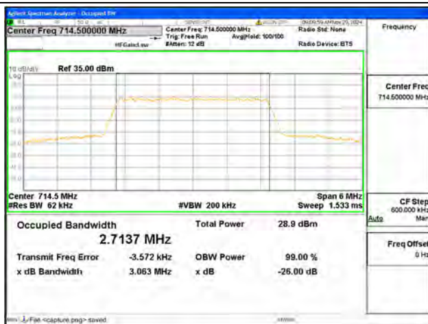
B12 / 3MHz / 16QAM/ High CH
