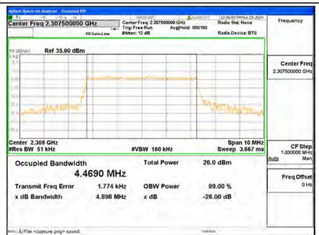
B40-1 / 5MHz / 16QAM/ Low CH
