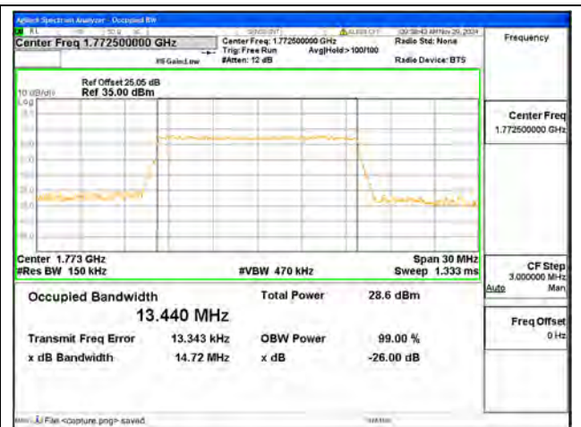
B66 / 15MHz / 16QAM/ High CH
