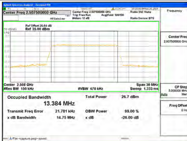
B7 / 15MHz / 64QAM/ Low CH
