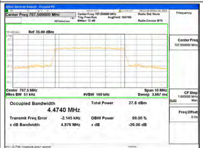
B12 / 5MHz / 64QAM/ Mid CH
