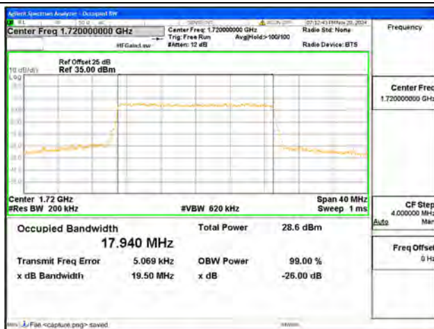
B4 / 20MHz / 16QAM/ Low CH
