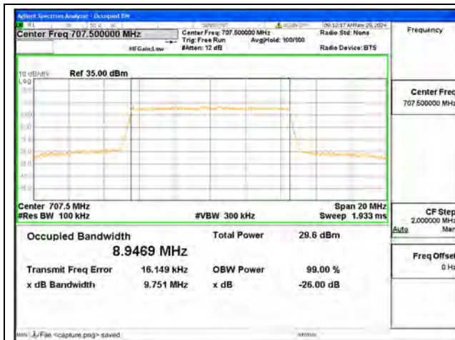
B12 / 10MHz / QPSK/ Mid CH
