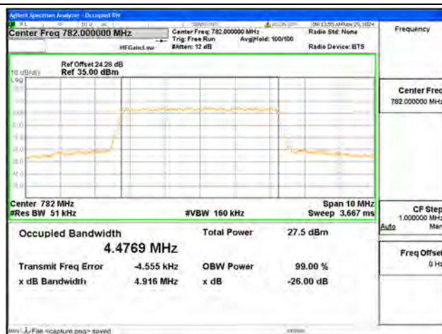
B13 / 5MHz / 16QAM/ Mid CH
