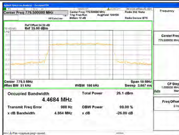
B13 / 5MHz / 64QAM/ Low CH
