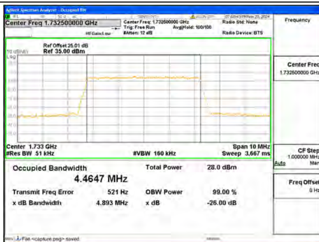
B4 / 5MHz / 16QAM/ Mid CH
