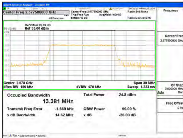
B38 / 15MHz / 64QAM/ Low CH
