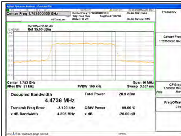
B4 / 5MHz / QPSK/ High CH
