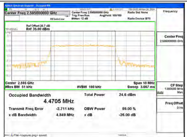
B38 / 5MHz / 64QAM/ Mid CH
