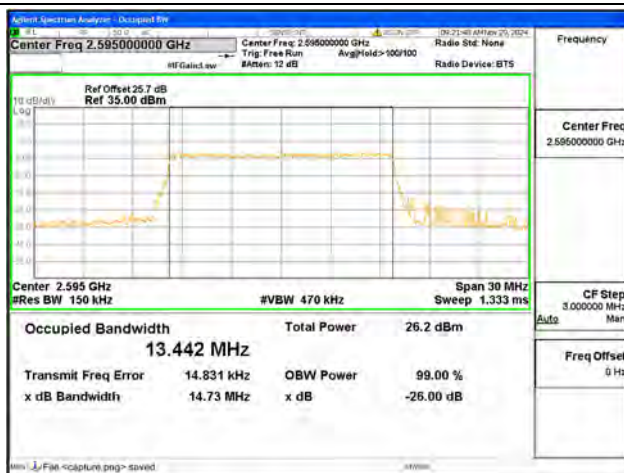
B38 / 15MHz / 16QAM/ Mid CH
