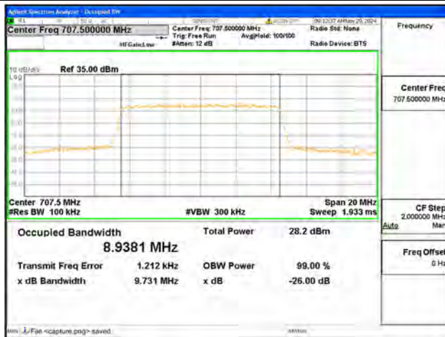
B12 / 10MHz / 64QAM/ Mid CH
