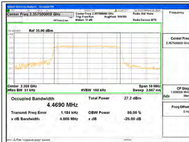
B40-2 / 5MHz / QPSK/ High CH
