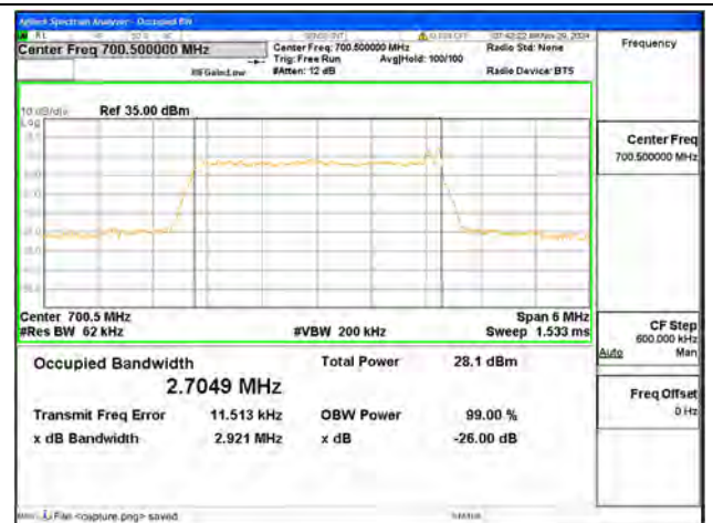
B12 / 3MHz / 64QAM/ Low CH
