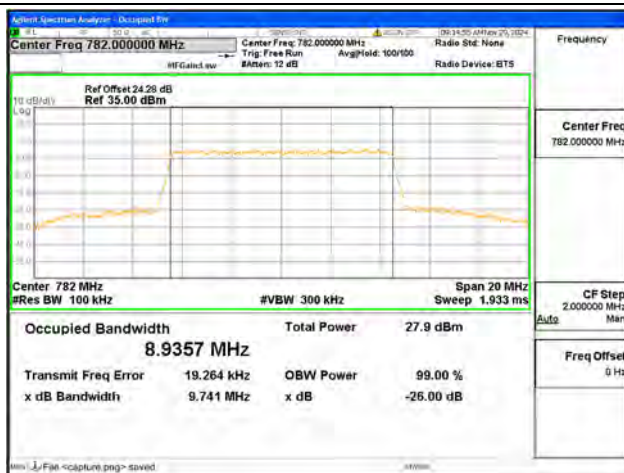
B13 / 10MHz / 16QAM/ Mid CH
