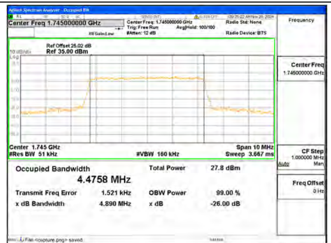
B66 / 5MHz / 64QAM/ Mid CH
