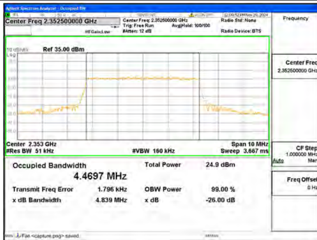
B40-2 / 5MHz / 64QAM/ Low CH
