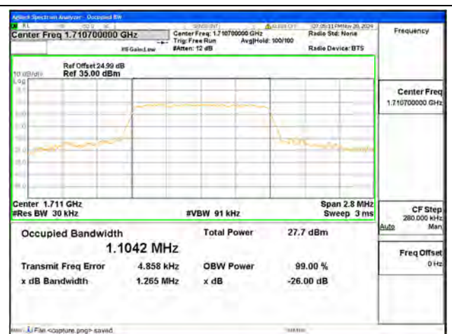
B4 / 1.4MHz / 16QAM/ Low CH
