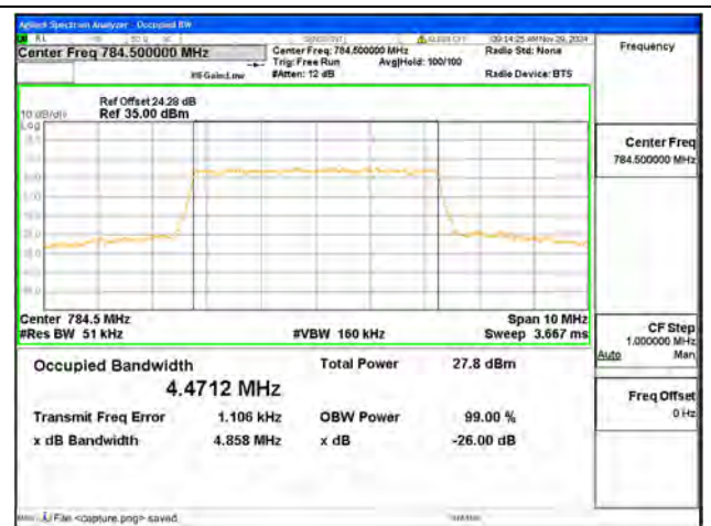
B13 / 5MHz / 16QAM/ High CH
