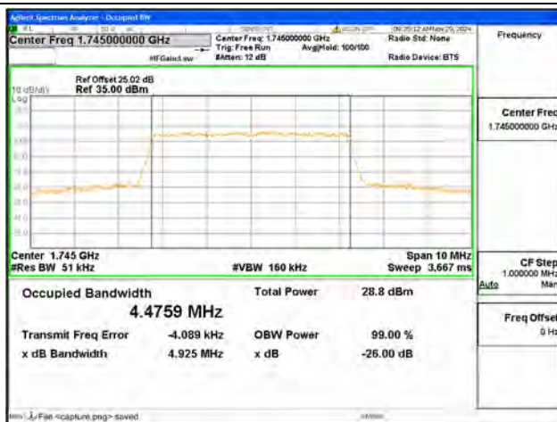
B66 / 5MHz / 16QAM/ Mid CH
