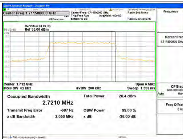
B4 / 3MHz / 16QAM/ Low CH
