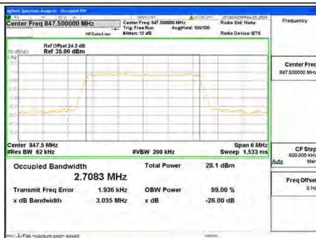
B5 / 3MHz / 64QAM/ High CH
