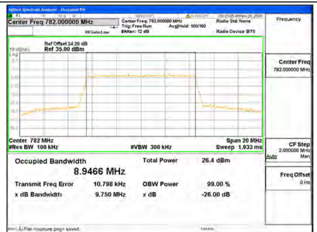
B13 / 10MHz / 64QAM/ Mid CH
