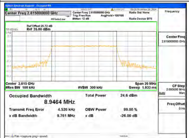
B38 / 10MHz / 64QAM/ High CH
