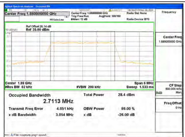
B2 / 3MHz / 16QAM/ Mid CH
