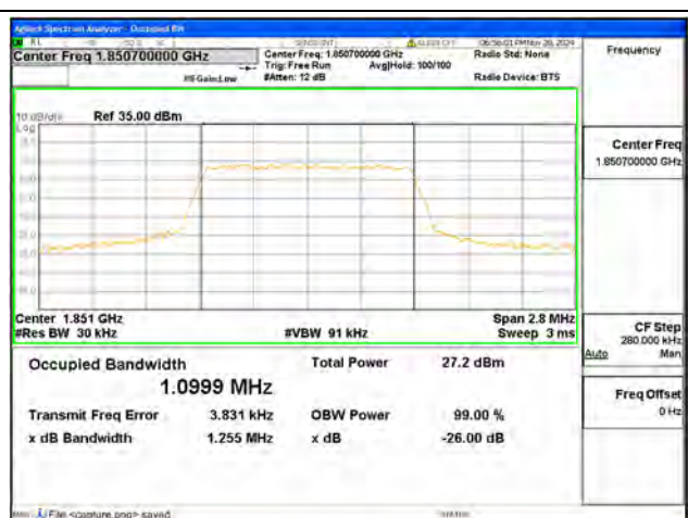
B2 / 1.4MHz / 16QAM/ Low CH
