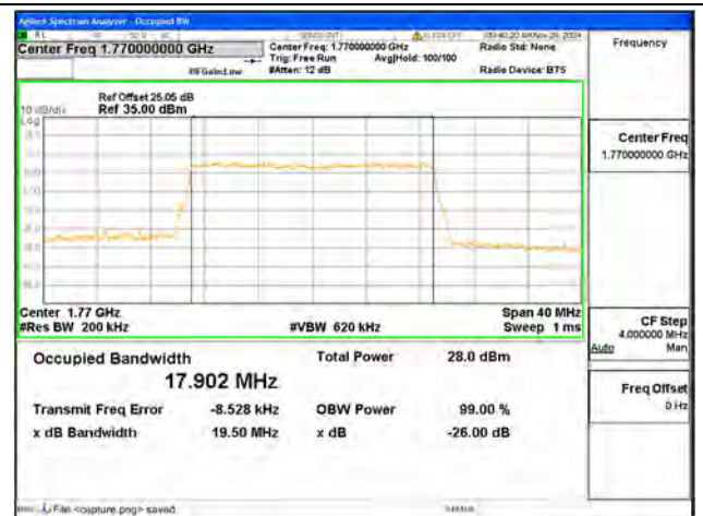
B66 / 20MHz / 64QAM/ High CH
