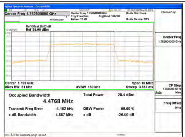
B4 / 5MHz / 16QAM/ High CH
