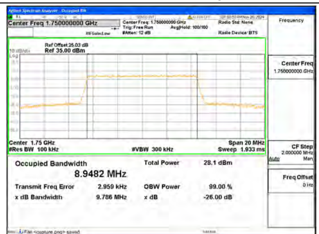
B4 / 10MHz / 64QAM/ High CH
