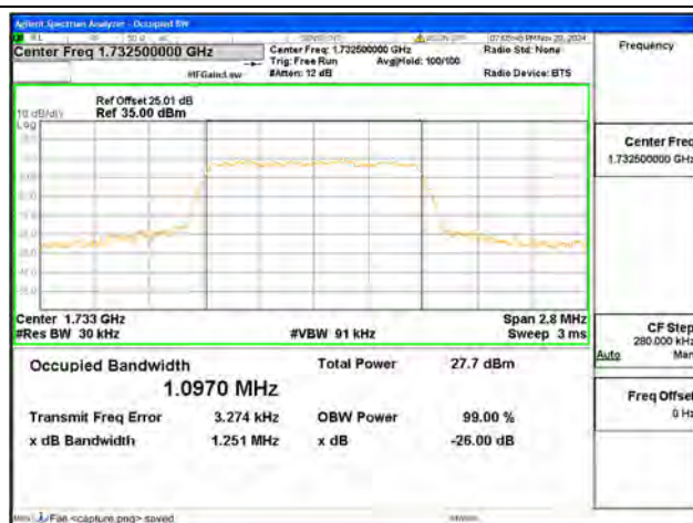
B4 / 1.4MHz / 16QAM/ Mid CH
