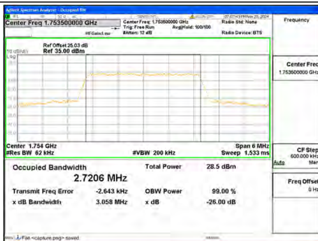
B4 / 3MHz / 16QAM/ High CH
