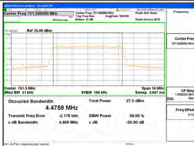
B12 / 5MHz / 64QAM/ Low CH
