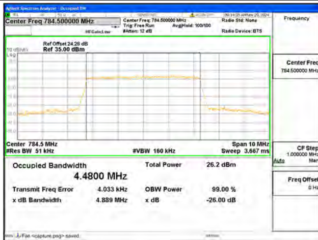
B13 / 5MHz / 64QAM/ High CH
