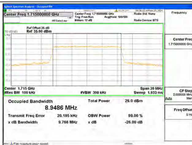
B66 / 10MHz / 16QAM/ Low CH
