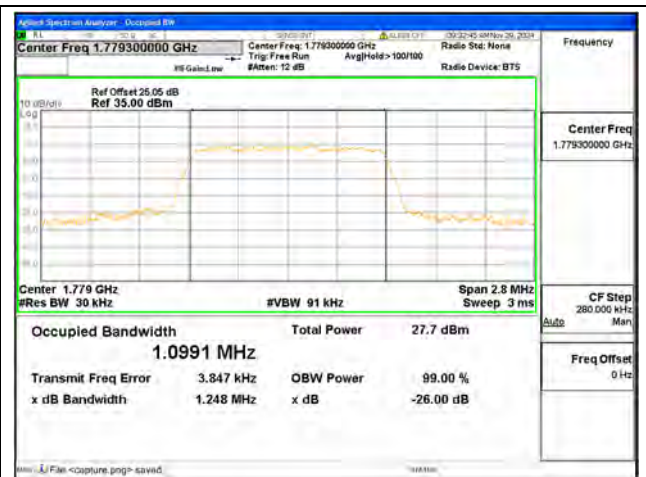
B66 / 1.4MHz / 16QAM/ High CH
