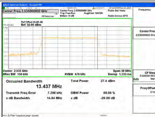
B7 / 15MHz / 16QAM/ Mid CH
