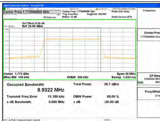
B66 / 10MHz / 16QAM/ High CH
