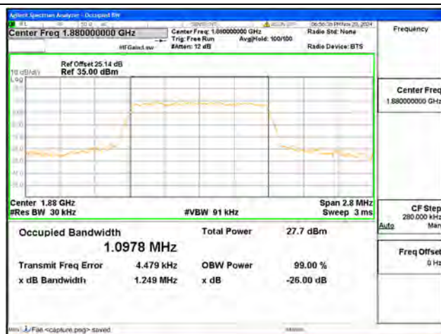
B2 / 1.4MHz / 16QAM/ Mid CH
