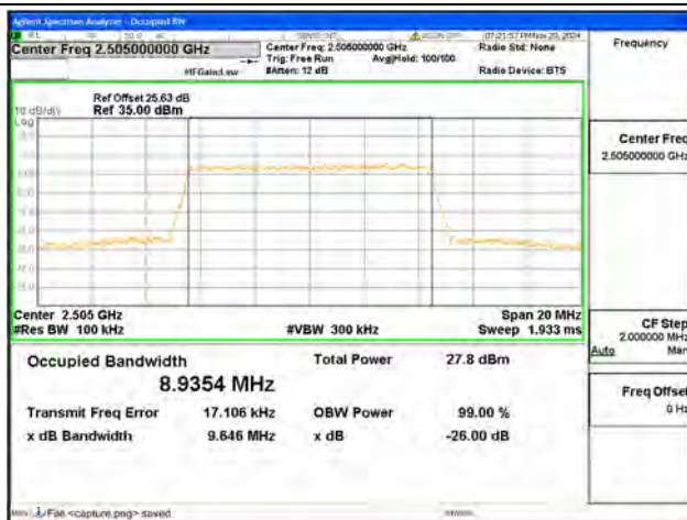
B7 / 10MHz / 16QAM/ Low CH
