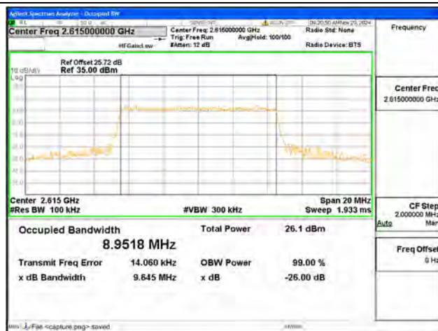
B38 / 10MHz / 16QAM/ High CH
