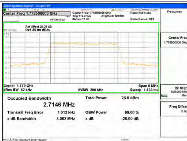
B66 / 3MHz / 16QAM/ High CH
