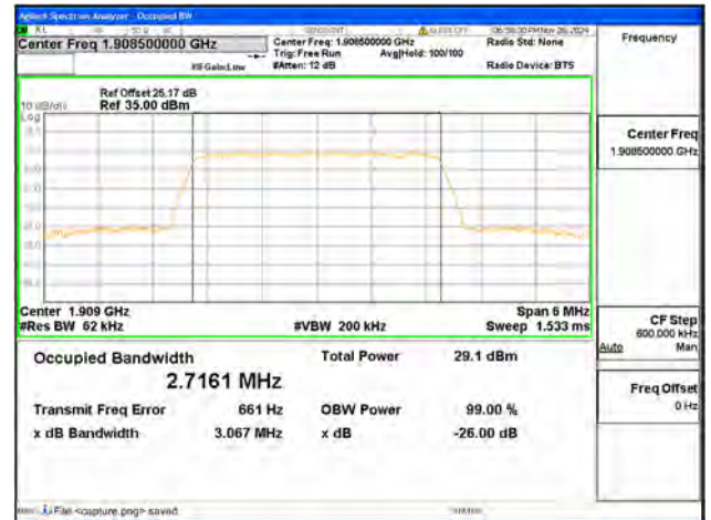
B2 / 3MHz / QPSK/ High CH
