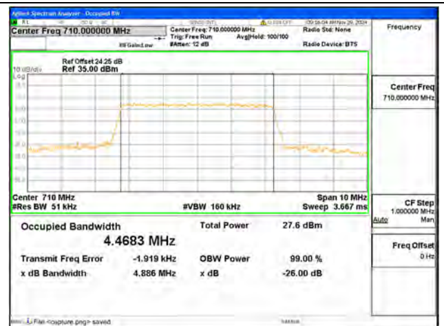
B17 / 5MHz / 64QAM/ Mid CH
