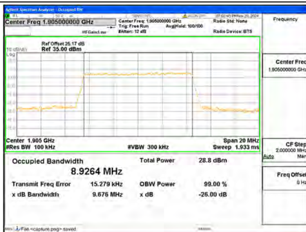
B2 / 10MHz / 16QAM/ High CH
