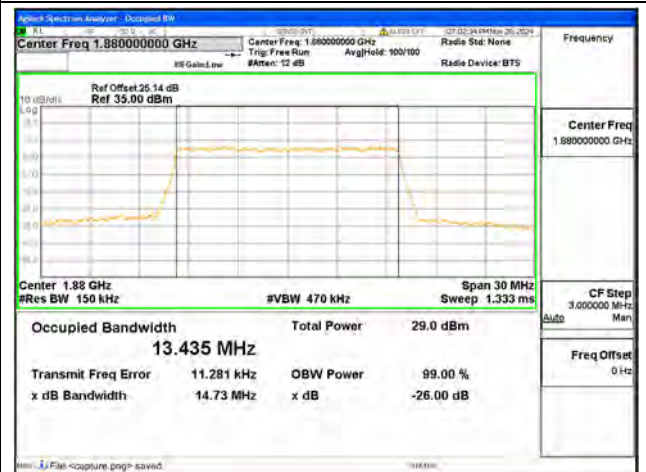
B2 / 15MHz / QPSK/ Mid CH
