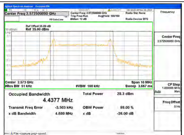
B38 / 5MHz / 16QAM/ Low CH
