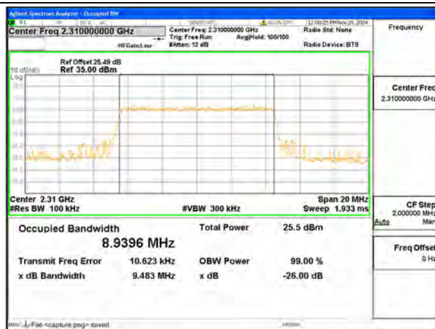
B40-1 / 10MHz / 16QAM/ Mid CH
