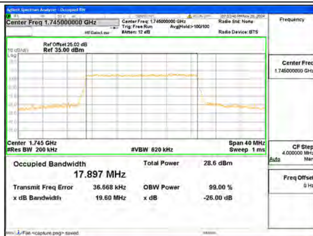
B4 / 20MHz / 16QAM/ High CH
