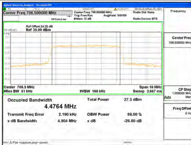
B17 / 5MHz / 64QAM/ Low CH
