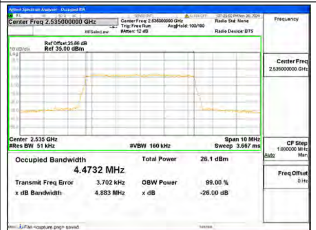
B7 / 5MHz / 64QAM/ Mid CH
