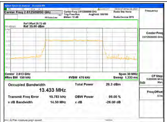
B38 / 15MHz / 16QAM/ High CH
