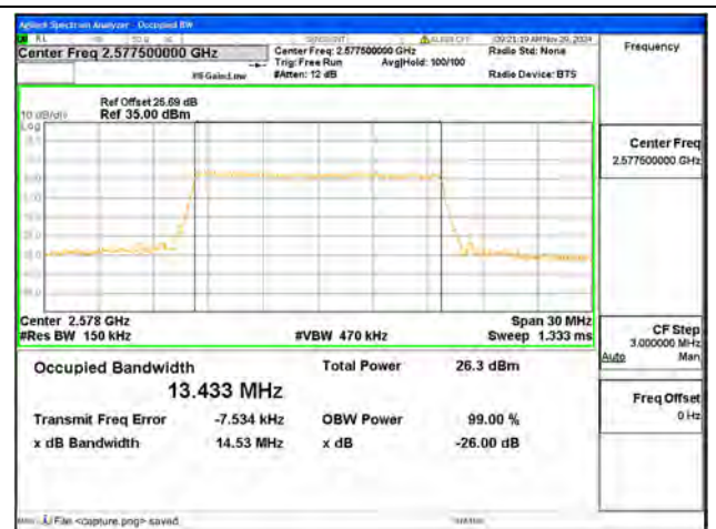
B38 / 15MHz / 16QAM/ Low CH
