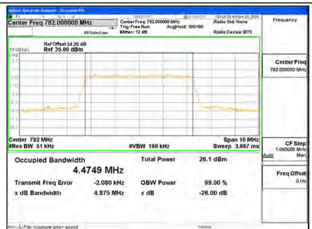
B13 / 5MHz / 64QAM/ Mid CH
