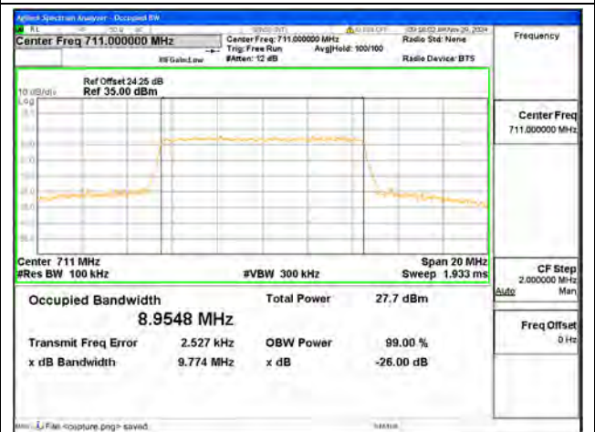
B17 / 10MHz / 64QAM/ High CH
