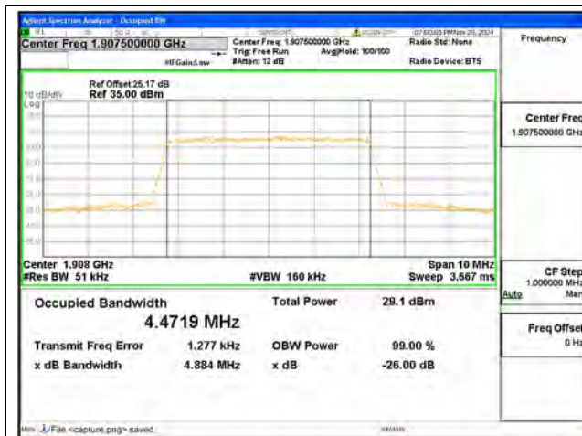
B2 / 5MHz / QPSK/ High CH
