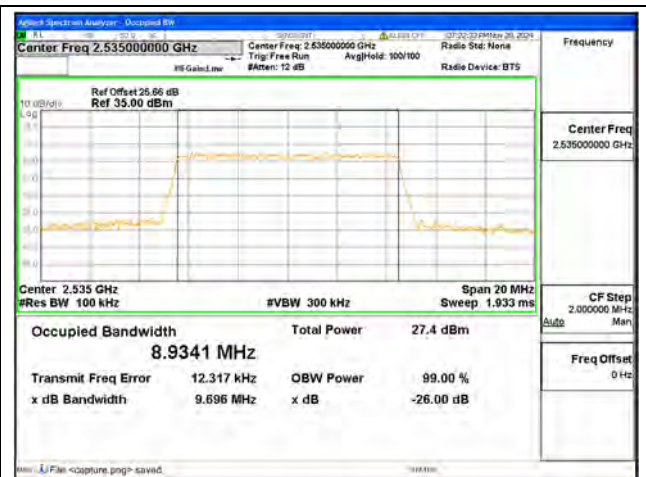
B7 / 10MHz / 16QAM/ Mid CH
