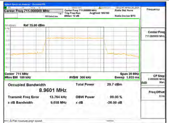
B12 / 10MHz / QPSK/ High CH
