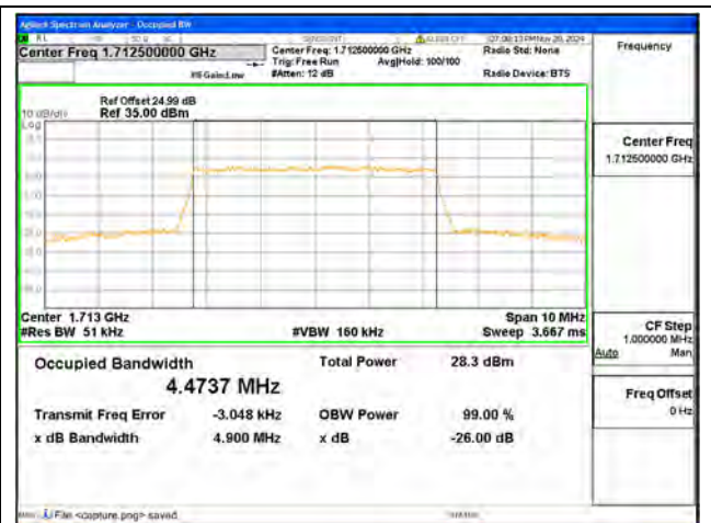
B4 / 5MHz / 16QAM/ Low CH
