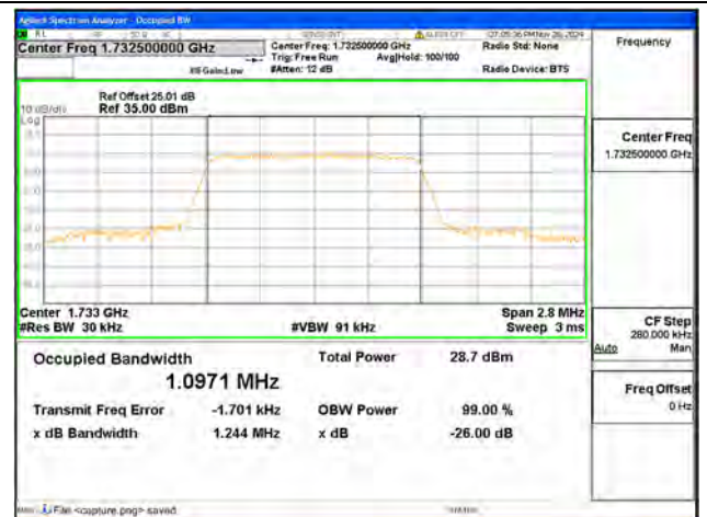
B4 / 1.4MHz / QPSK/ Mid CH
