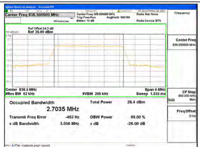
B5 / 3MHz / 16QAM/ Mid CH
