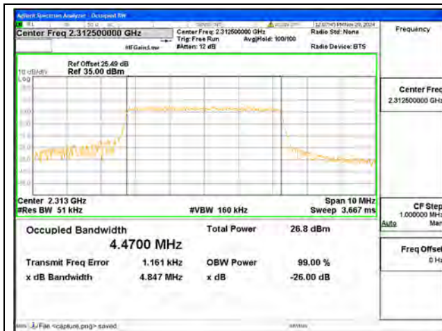
B40-1 / 5MHz / QPSK/ High CH
