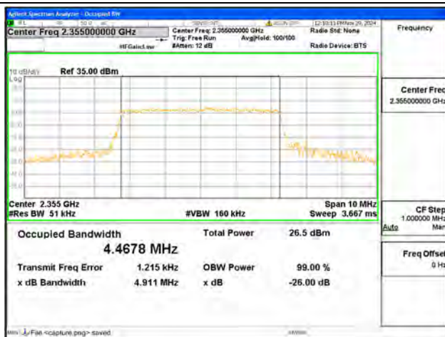
B40-2 / 5MHz / 16QAM/ Mid CH
