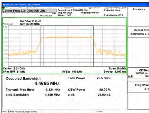
B40-1 / 5MHz / 16QAM/ Mid CH
