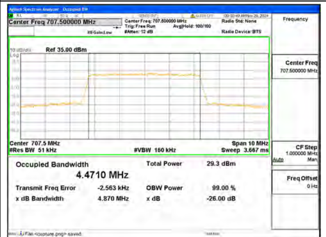
B12 / 5MHz / QPSK/ Mid CH
