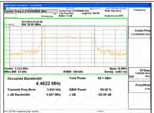
B40-1 / 5MHz / 16QAM/ High CH
