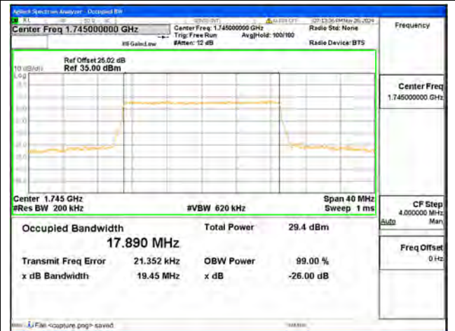
B4 / 20MHz / QPSK/ High CH
