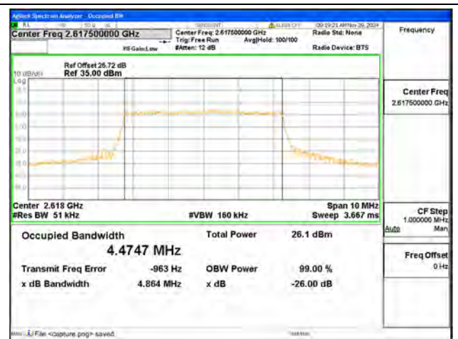
B38 / 5MHz / 16QAM/ High CH
