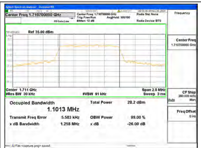
B66 / 1.4MHz / 16QAM/ Low CH
