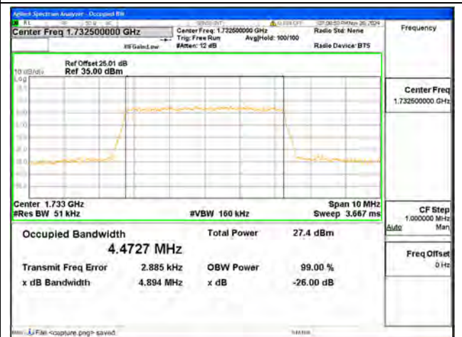
B4 / 5MHz / 64QAM/ Mid CH
