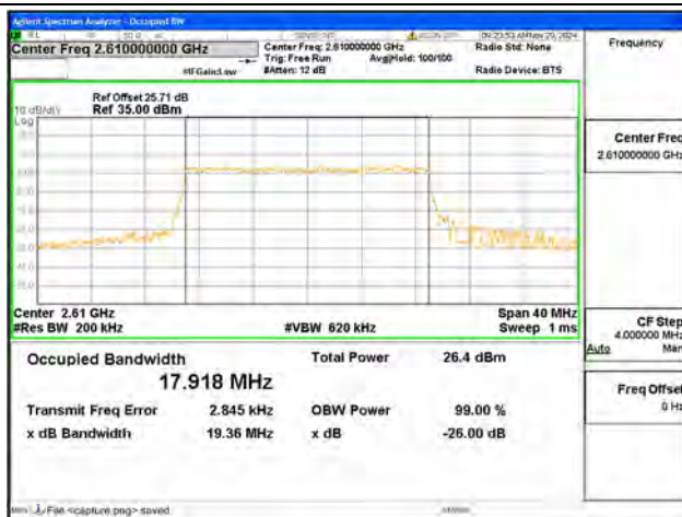
B38 / 20MHz / 16QAM/ High CH
