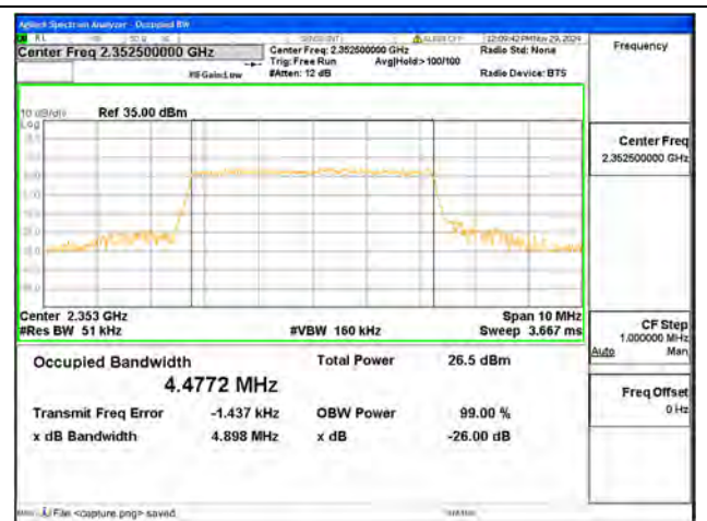
B40-2 / 5MHz / 16QAM/ Low CH
