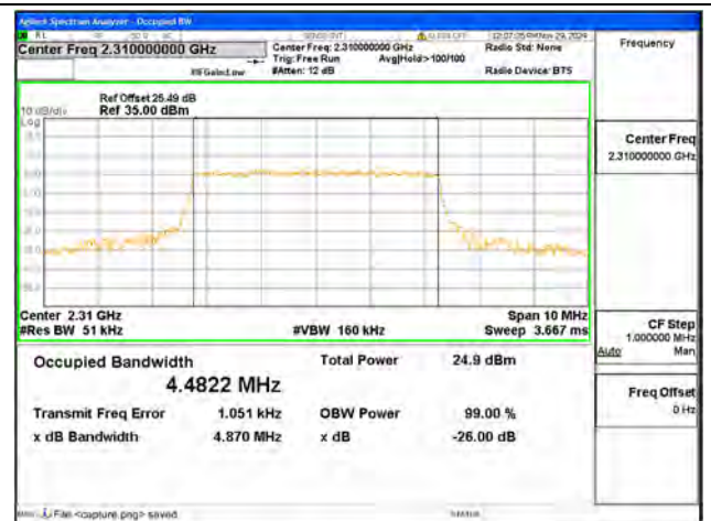
B40-1 / 5MHz / 64QAM/ Mid CH
