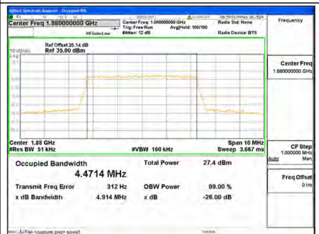
B2 / 5MHz / 64QAM/ Mid CH
