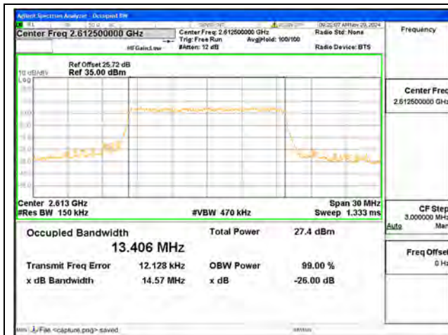
B38 / 15MHz / QPSK/ High CH
