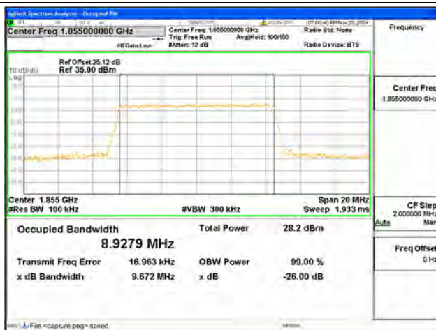
B2 / 10MHz / 16QAM/ Low CH
