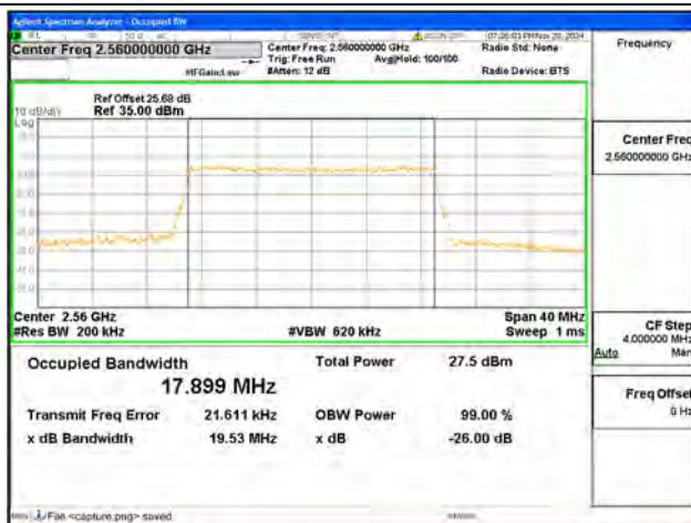
B7 / 20MHz / 16QAM/ High CH
