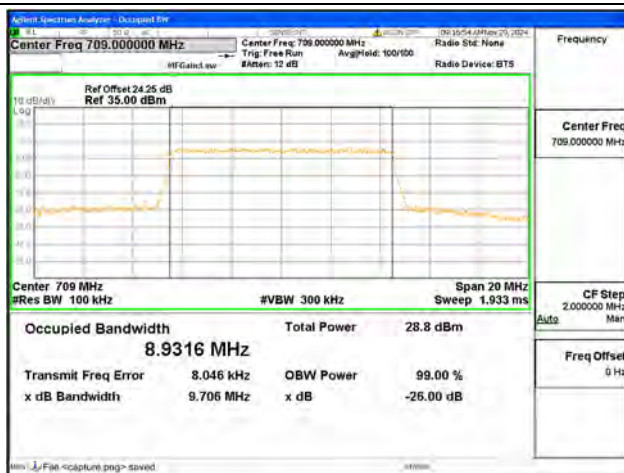
B17 / 10MHz / 16QAM/ Low CH
