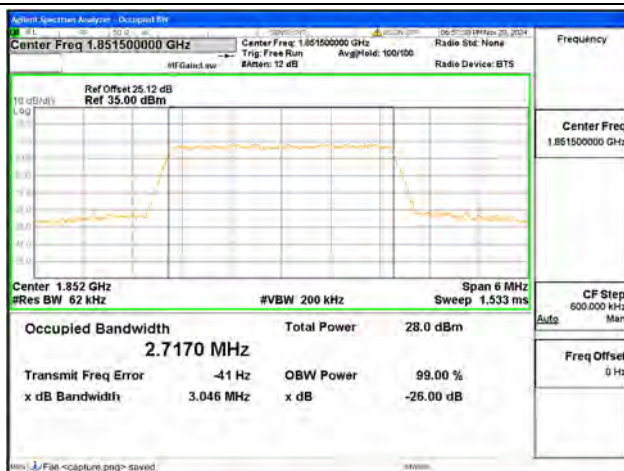
B2 / 3MHz / 16QAM/ Low CH
