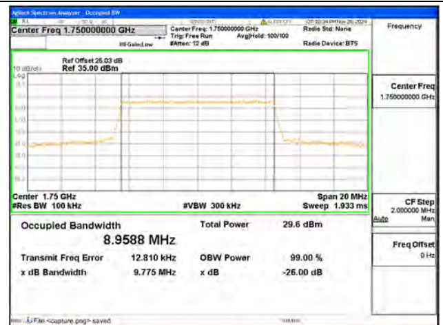
B4 / 10MHz / QPSK/ High CH
