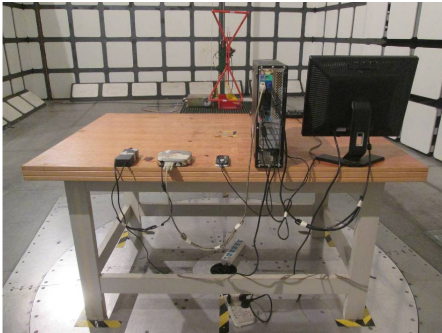
Radiated Emissions – Rear View (Below 1 GHz)
