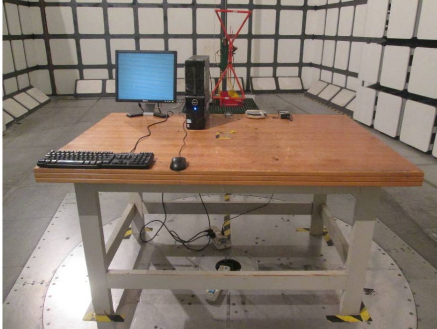
Radiated Emissions – Front View (Below 1 GHz)
