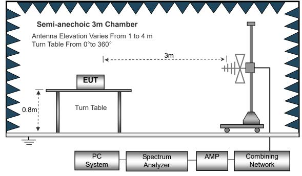
(C) Radiated Emission Test-Up Frequency Above 1GHz
