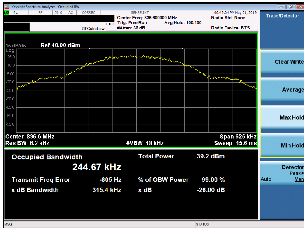
Plot 7-1. Occupied Bandwidth Plot (Cellular GPRS Mode)
