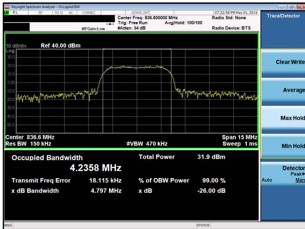
Plot 7-5. Occupied Bandwidth Plot (Cellular WCDMA Mode)
