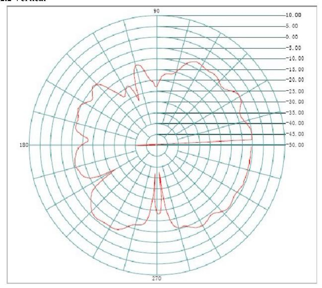
Frequency(MHZ): 2480 Antenna Polarity: Vertical
