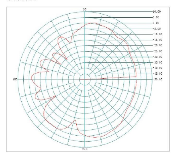
Frequency(MHZ): 2402 Antenna Polarity: Horizontal
