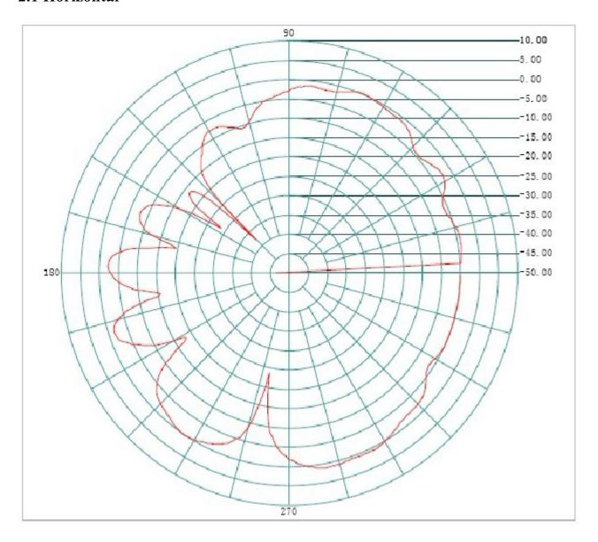
Frequency(MHZ): 2480 Antenna Polarity: Horizontal
