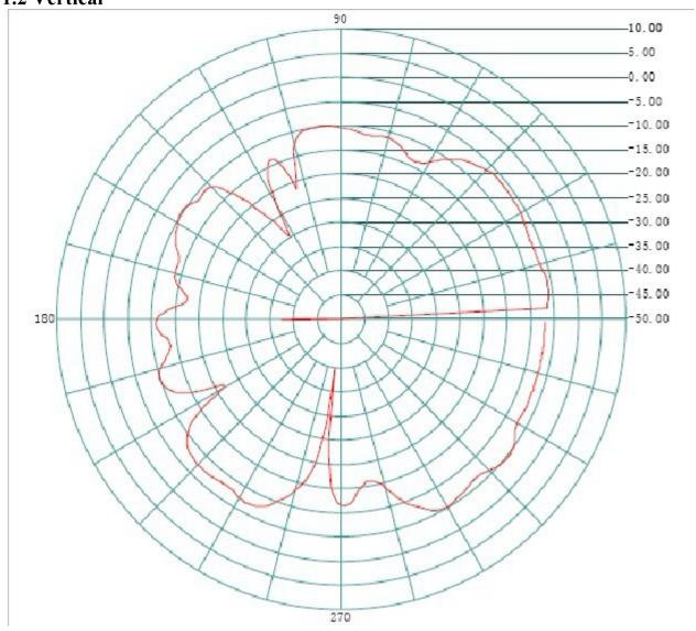
Frequency(MHZ): 2402 Antenna Polarity: Vertical
