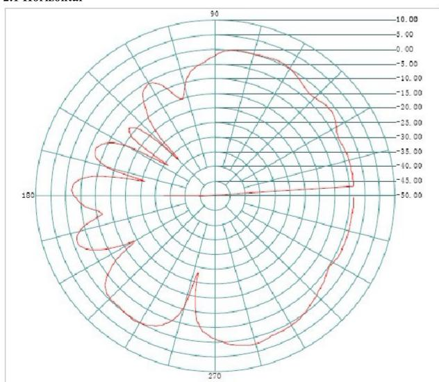
Frequency(MHZ): 2441 Antenna Polarity: Horizontal
