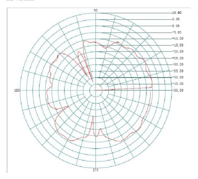
Frequency(MHZ): 2441 Antenna Polarity: Vertical
