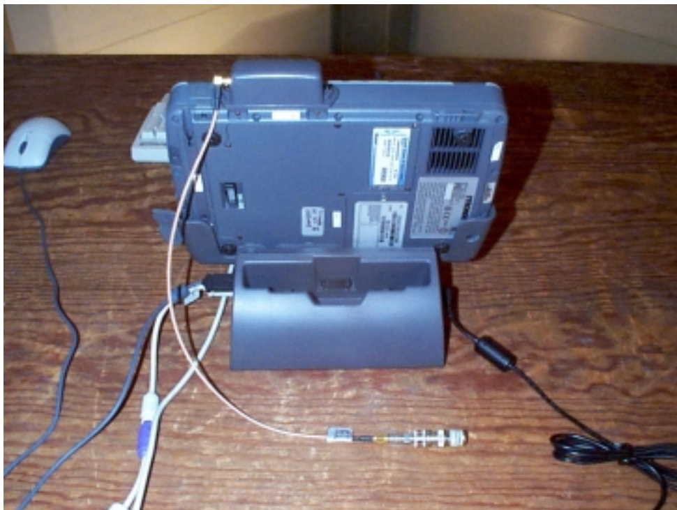
AirCard 555 antenna removed and a resistive 50 ohm load connected during the radiated spurious and harmonics.
