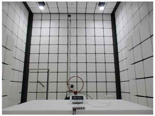
Radiated Emission Set up Photos (Below 1GHz)
