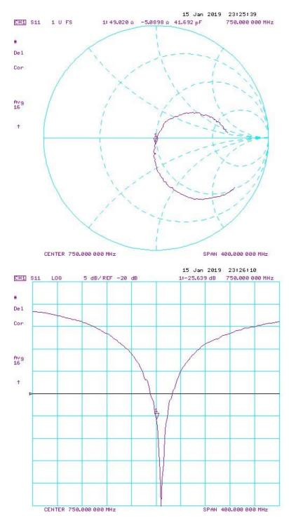
Impedance & Return-Loss Measurement Plot for Body TSL
