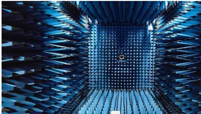
Figure 2: Geometry of Anechoic Chamber for Radiation patterns.
