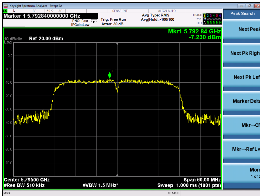
TEST PLOT OF SPECTRAL DENSITY FOR 5795MHz AT CHAIN 3
