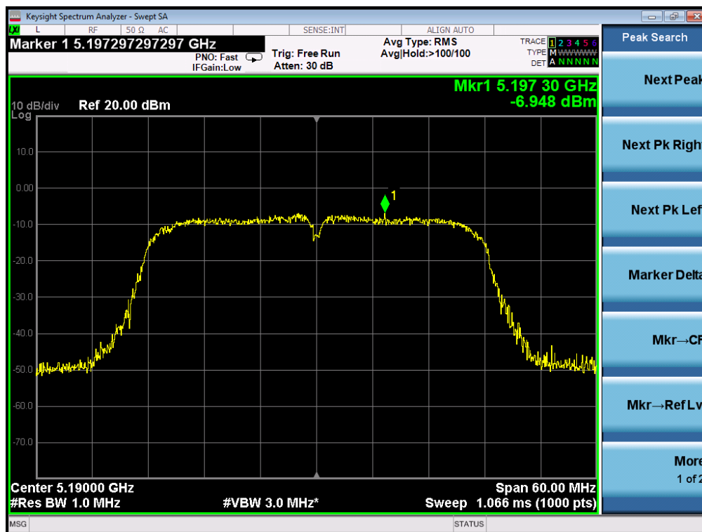
TEST PLOT OF SPECTRAL DENSITY FOR 5190MHz AT CHAIN 3
