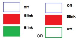
In advertising mode, either the Green and Red LED or only the Red LED blinks at a rate of 2X per second. If the green LED is blinking, this means that the module is in pairing mode and that it will accept a new bond.
