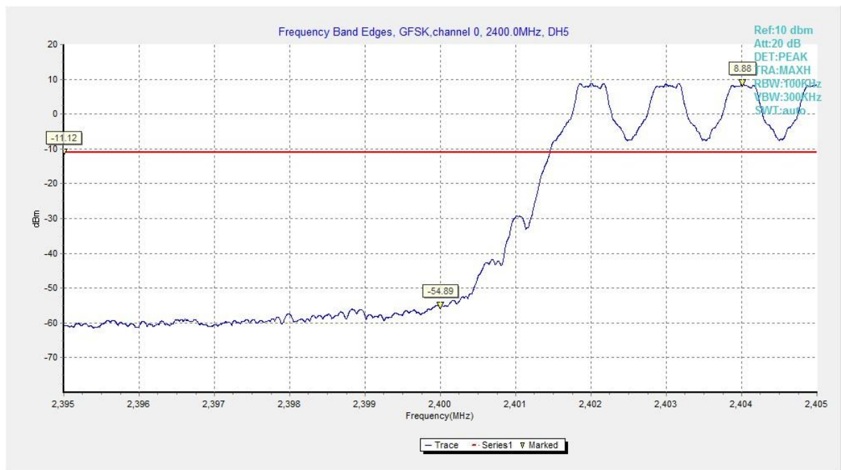
Fig. 1 Band Edges (GFSK, Ch 0, Hopping ON)
