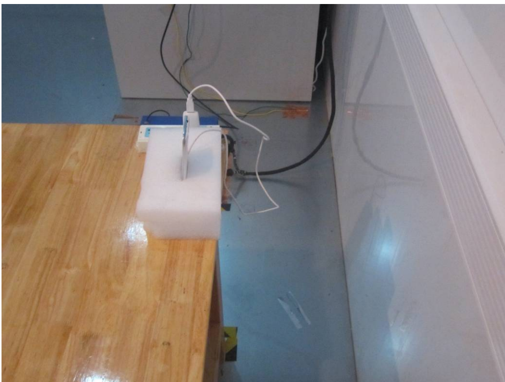
Conducted Emissions Test Setup Side View
