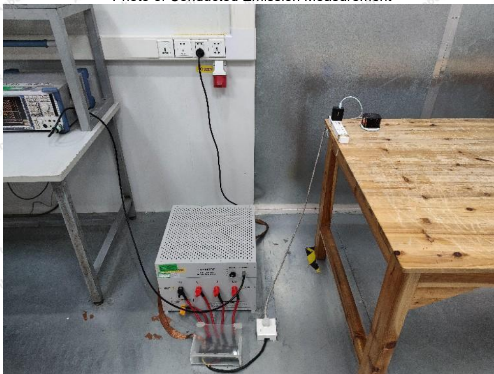
Photo of Conducted Emission Measurement
