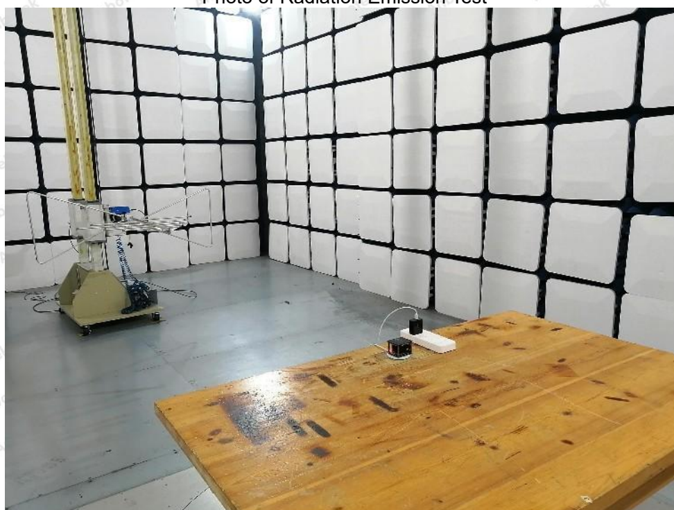
Photo of Radiation Emission Test
