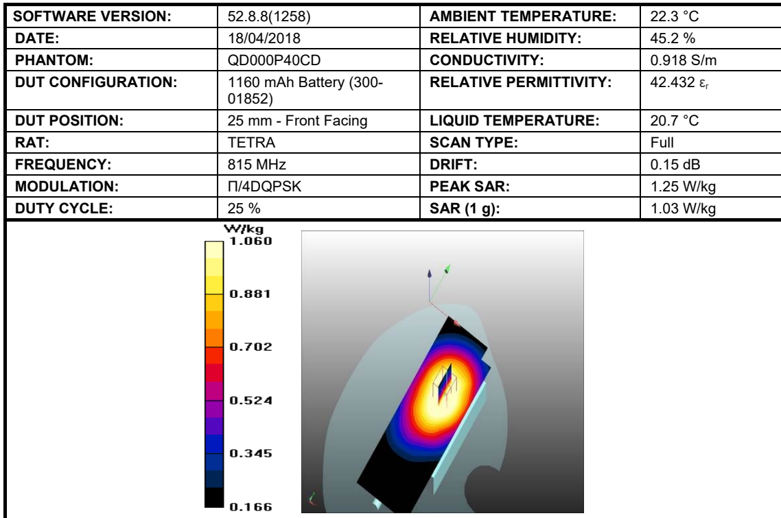
Figure 21: SAR Head Testing Results for the SC2128 TETRA Radio at 815 MHz.
