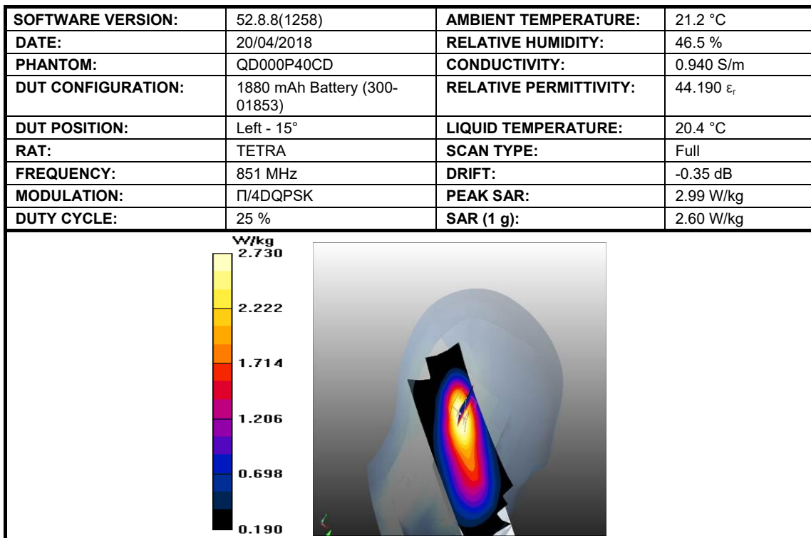
Figure 18: SAR Head Testing Results for the SC2128 TETRA Radio at 851 MHz.
