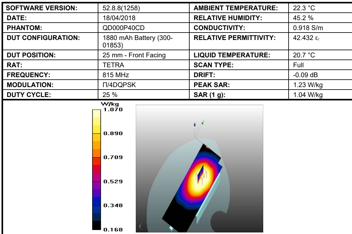
Figure 22: SAR Head Testing Results for the SC2128 TETRA Radio at 815 MHz.
