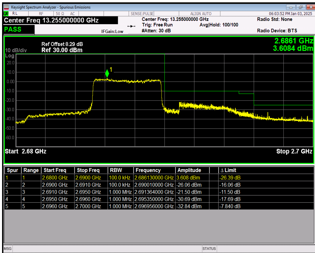
Band41 16QAM BW=5MHz Channel=41565 RB Size=1 Position=#0
