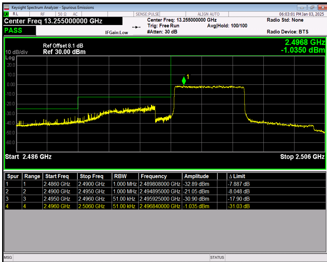
Band41 16QAM BW=5MHz Channel=39675 RB Size=1 Position=#0
