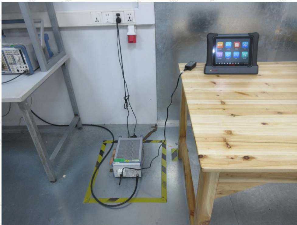
Photo of Power Line Conducted Emission Test
