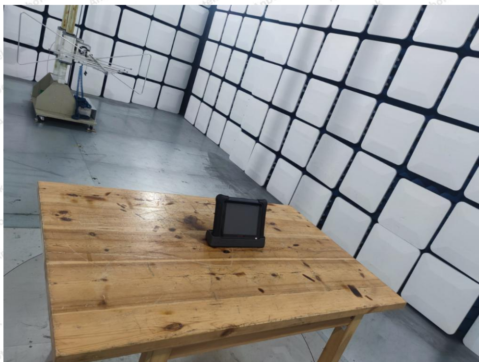
Photo of Radiation Emission Test
