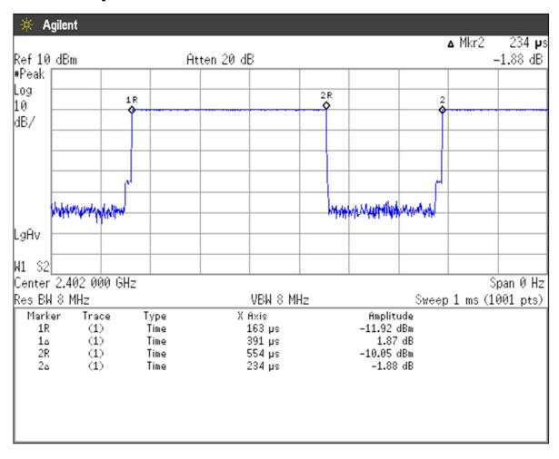
Duty Cycle = Ton / (Ton + Toff) =  $391[\mu s] / (391[\mu s] + 234[\mu s]) = 62.56[\%]$
